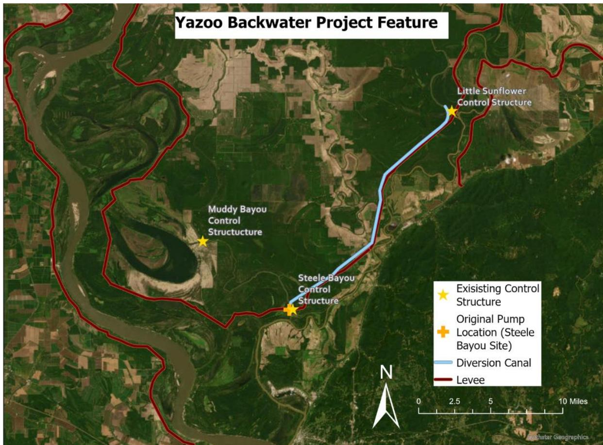
Figure 2-5. The flood control projects in the Yazoo Backwater Area.
