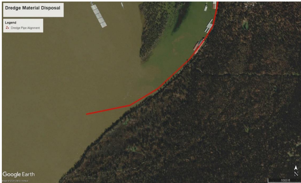
Figure 6-4. Dredge Pipe Alignment and Extent of Disposal.
