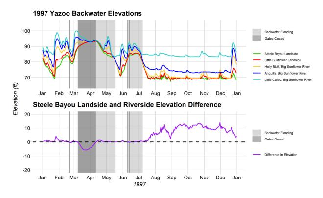
Figure 2-18. The Yazoo Backwater elevations and the Steele Bayou landside and riverside elevation differences for the 1997 Yazoo Backwater flood
