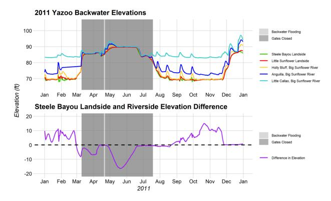
Figure 2-29. The Yazoo Backwater elevations and the Steele Bayou landside and riverside elevation differences for the 2011 Yazoo Backwater flood.
