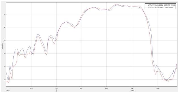
Figure 2-71. Little Sunflower Control Structure Landside 2019 Calibration.
