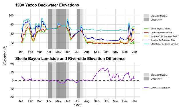
Figure 2-19. The Yazoo Backwater elevations and the Steele Bayou landside and riverside elevation differences for the 1998 Yazoo Backwater flood.
