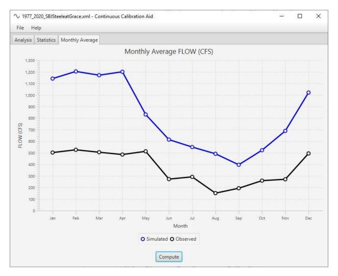
Figure 2-49. Steele Bayou at Grace Monthly Flow Comparison.
