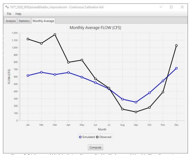
Figure 2-54. Improved Model - Quiver River at Doddsville Improved Monthly Flow Comparison.
