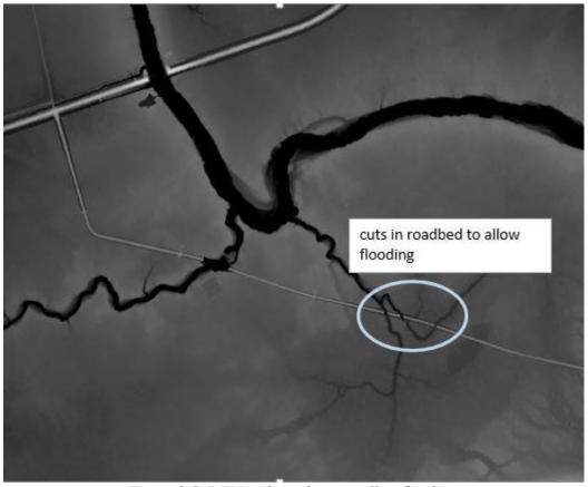
Figure 2-3. DEM with roads cut to allow flooding.
