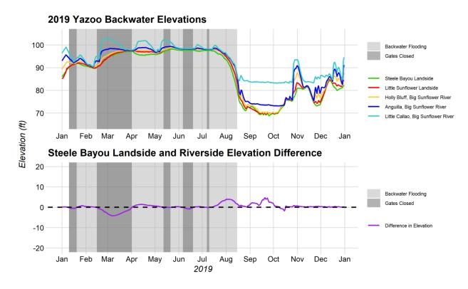
Figure 2-36. The Yazoo Backwater elevations and the Steele Bayou landside and riverside elevation differences for the 2019 Yazoo Backwater flood.
