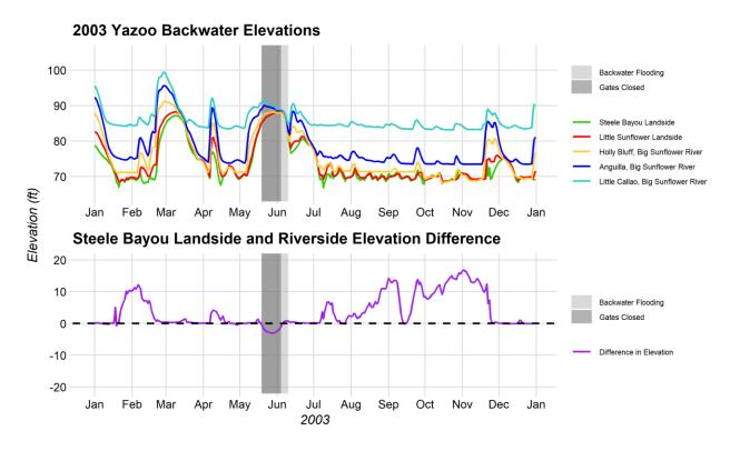
Figure 2-22. The Yazoo Backwater elevations and the Steele Bayou landside and riverside elevation differences for the 2003 Yazoo Backwater flood.
