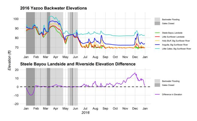
Figure 2-33. The Yazoo Backwater elevations and the Steele Bayou landside and riverside elevation differences for the 2016 Yazoo Backwater flood.
