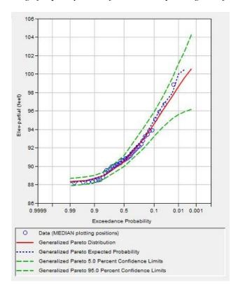
Figure 2-107. The stage-frequency curves for the upper ponding area for base conditions.
