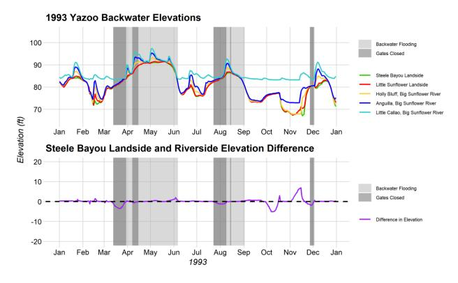
Figure 2-17. The Yazoo Backwater elevations and the Steele Bayou landside and riverside elevation differences for the 1993 Yazoo Backwater flood.
