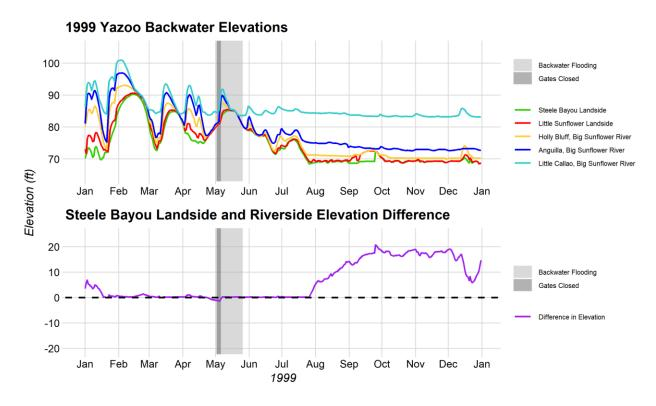
Figure 2-20. The Yazoo Backwater elevations and the Steele Bayou landside and riverside elevation differences for the 1999 Yazoo Backwater flood.
