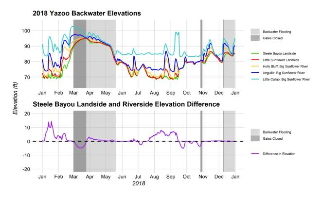
Figure 2-35. The Yazoo Backwater elevations and the Steele Bayou landside and riverside elevation differences for the 2018 Yazoo Backwater flood.
