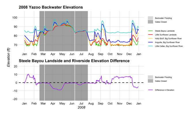
Figure 2-26. The Yazoo Backwater elevations and the Steele Bayou landside and riverside elevation differences for the 2008 Yazoo Backwater flood.
