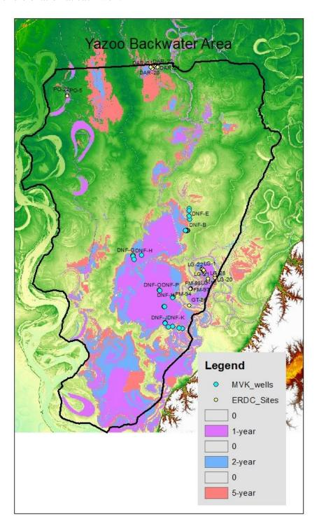
Figure 2-4. Shallow groundwater wells relative to flood frequency zones.
