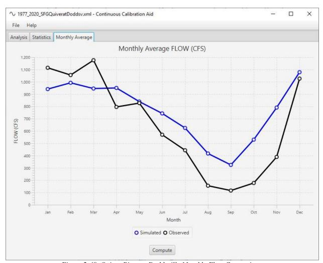
Figure 2-48. Quiver River at Doddsville Monthly Flow Comparison.
