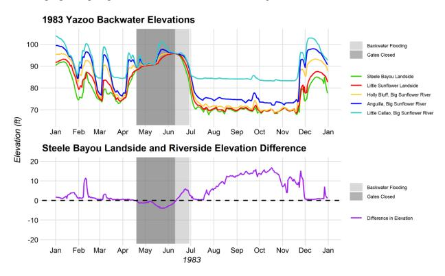
Figure 2-14. The Yazoo Backwater elevations and the Steele Bayou landside and riverside elevation differences for the 1983 Yazoo Backwater flood.
