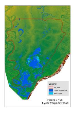
Figure 2-110. The FESM model 1-year frequency flood for base conditions and with-pump conditions.
