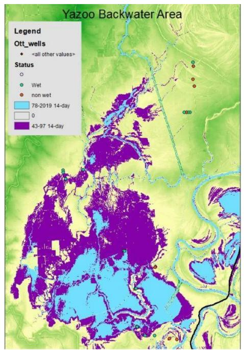
Figure 2-5. Shallow groundwater wells relative to flood duration zones.
