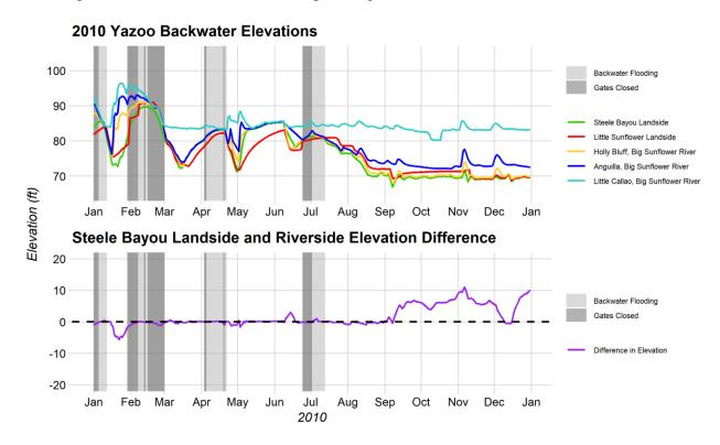
Figure 2-28. The Yazoo Backwater elevations and the Steele Bayou landside and riverside elevation differences for the 2010 Yazoo Backwater flood.
