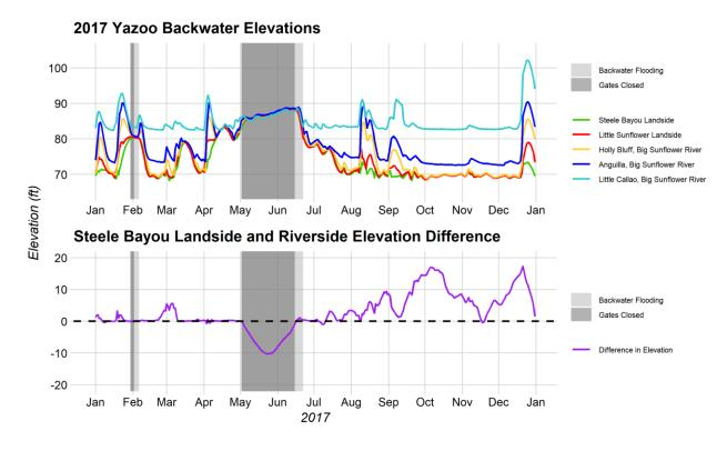
Figure 2-34. The Yazoo Backwater elevations and the Steele Bayou landside and riverside elevation differences for the 2017 Yazoo Backwater flood.
