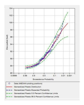
Figure 2-106. The stage-frequency curves for the lower ponding area for base conditions.
