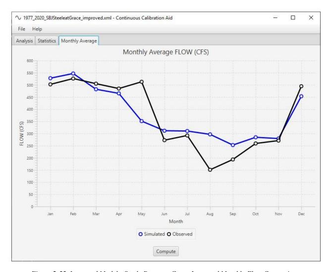
Figure 2-55. Improved Model - Steele Bayou at Grace Improved Monthly Flow Comparison.
