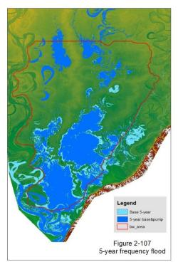
Figure 2-112. The FESM model 5-year frequency flood for base conditions and with-pump conditions.
