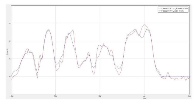
Figure 2-64. Steele Bayou Landside 2004 Calibration.
