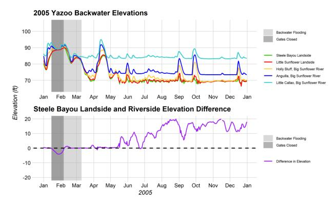
Figure 2-24. The Yazoo Backwater elevations and the Steele Bayou landside and riverside elevation differences for the 2005 Yazoo Backwater flood.
