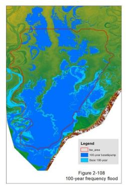
Figure 2-113. The FESM model 100-year frequency flood for base conditions and with-pump conditions.
