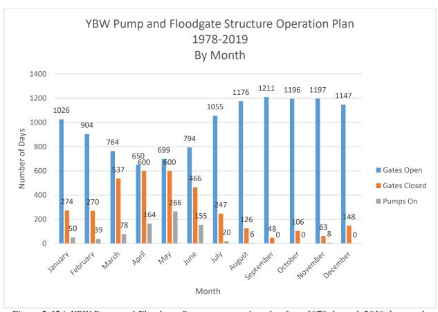
Figure 2-124. YBW Pump and Floodgate Structure operation plan from 1978 through 2019, by month.
