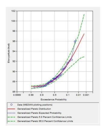
Figure 2-108. The stage-frequency curve for the lower ponding area for the proposed plan.
