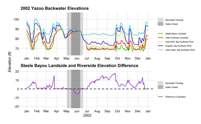
Figure 2-21. The Yazoo Backwater elevations and the Steele Bayou landside and riverside elevation differences for the 2002 Yazoo Backwater flood.
