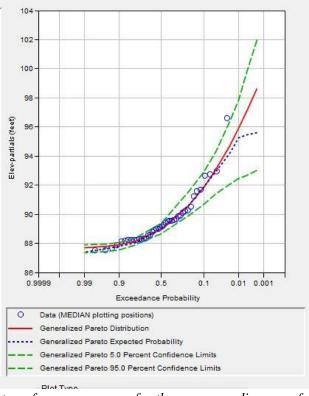
Figure 2-109. The stage-frequency curves for the upper ponding area for the proposed plan.
