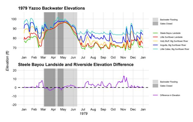
Figure 2-13. The Yazoo Backwater elevations and the Steele Bayou landside and riverside elevation differences for the 1979 Yazoo Backwater flood.
