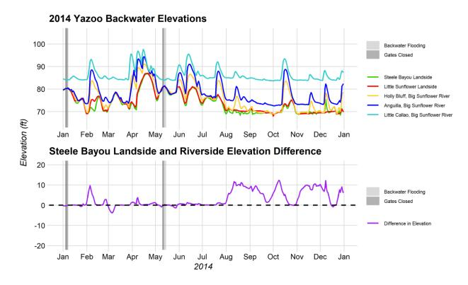
Figure 2-31. The Yazoo Backwater elevations and the Steele Bayou landside and riverside elevation differences for the 2014 Yazoo Backwater flood.
