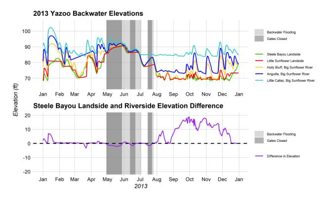
Figure 2-30. The Yazoo Backwater elevations and the Steele Bayou landside and riverside elevation differences for the 2013 Yazoo Backwater flood.
