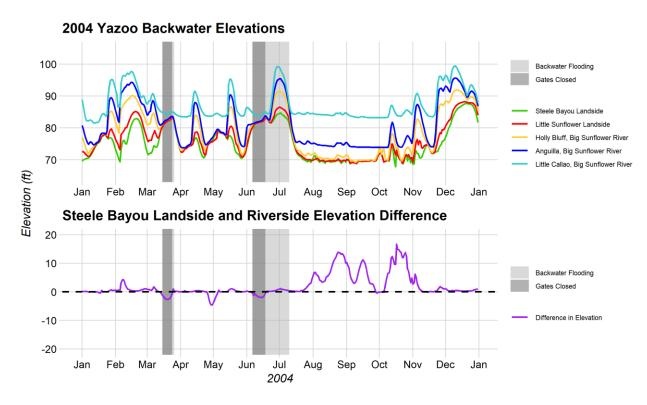
Figure 2-23. The Yazoo Backwater elevations and the Steele Bayou landside and riverside elevation differences for the 2004 Yazoo Backwater flood.
