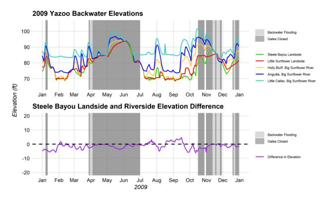
Figure 2-27. The Yazoo Backwater elevations and the Steele Bayou landside and riverside elevation differences for the 2009 Yazoo Backwater flood.
