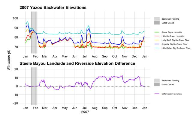
Figure 2-25. The Yazoo Backwater elevations and the Steele Bayou landside and riverside elevation differences for the 2007 Yazoo Backwater flood.
