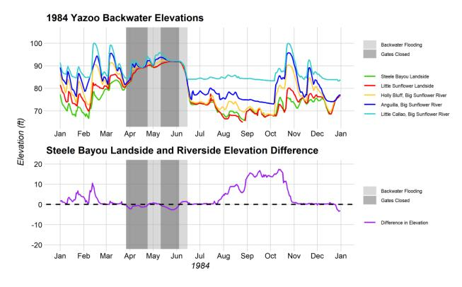
Figure 2-15. The Yazoo Backwater elevations and the Steele Bayou landside and riverside elevation differences for the 1984 Yazoo Backwater flood.
