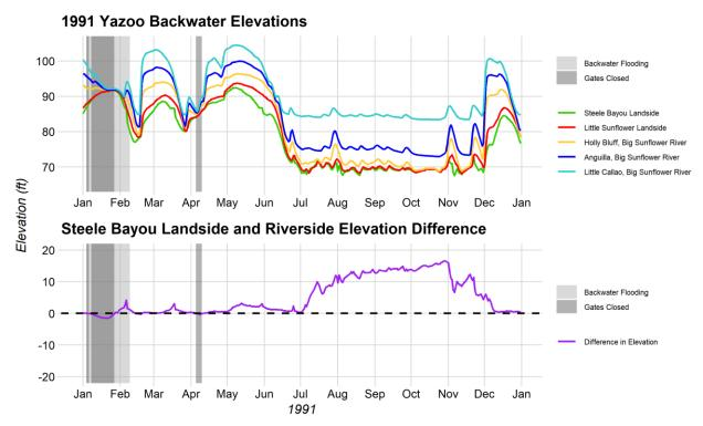
Figure 2-16. The Yazoo Backwater elevations and the Steele Bayou landside and riverside elevation differences for the 1991 Yazoo Backwater flood.
