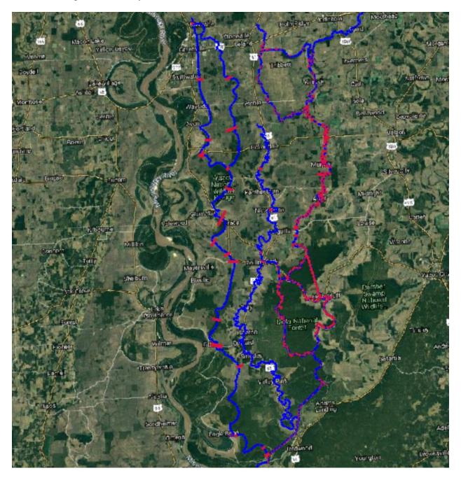
Figure 2-57. The cross sections for the Yazoo Study Area, indicated in red, along the centerlines of the rivers modeled, indicated in blue.
