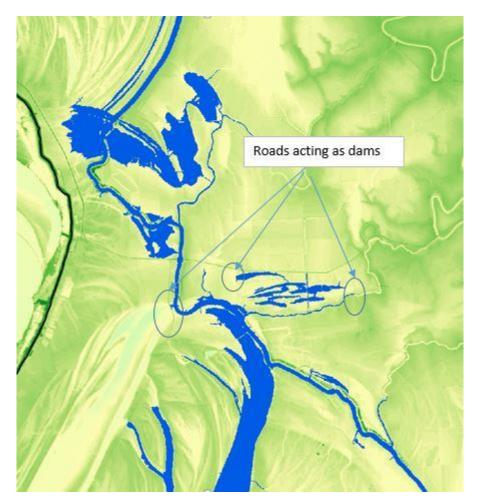
Figure 2-2. FESM simulation blocked by roads.
