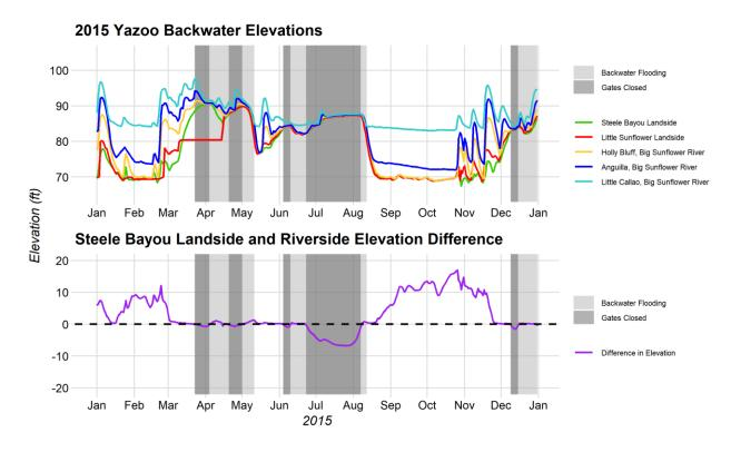
Figure 2-32. The Yazoo Backwater elevations and the Steele Bayou landside and riverside elevation differences for the 2015 Yazoo Backwater flood.
