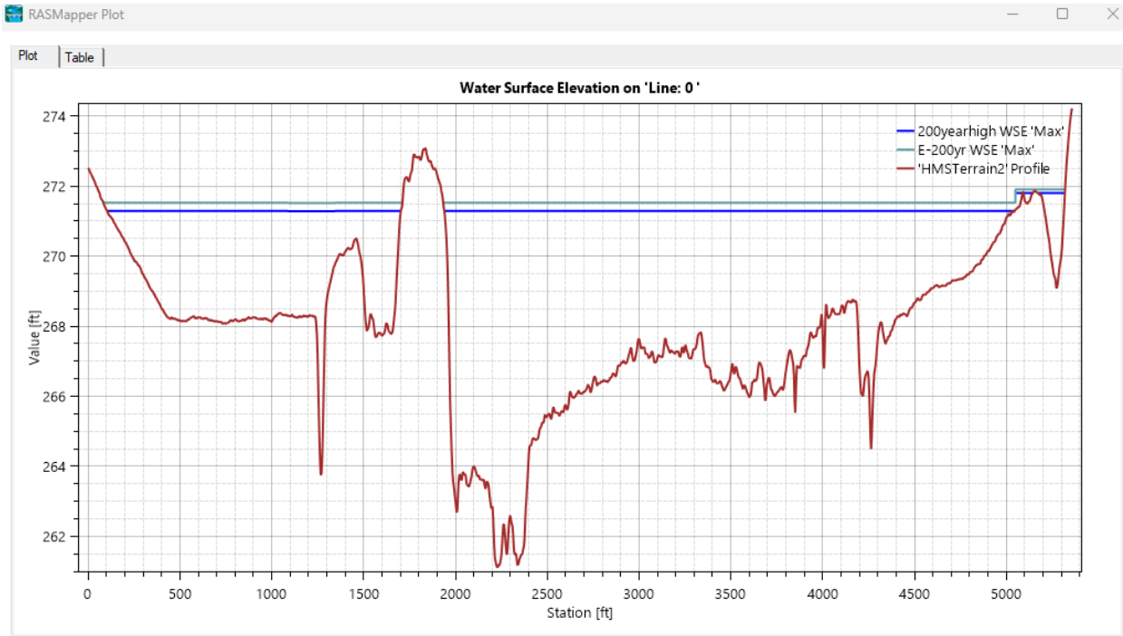
Figure 1-27. Caney Creek Levee Location, Existing Terrain, as compared to the 200-year Flood Elevations, with and without channel improvements
