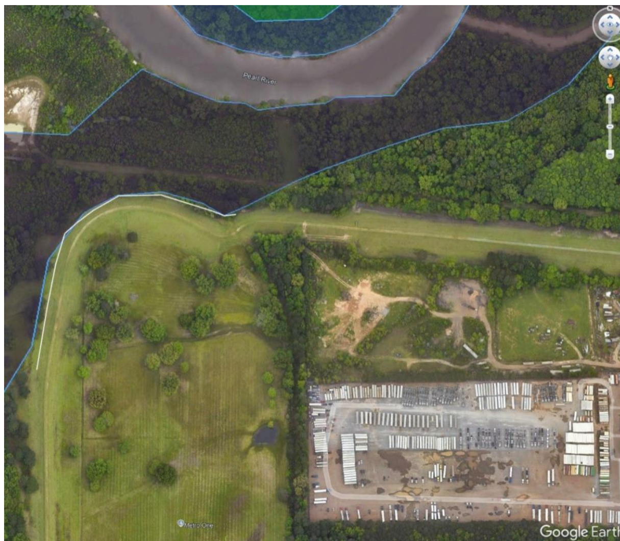
Figure 2-24. Work near Areas of HTRW Concern, Channel Overbank Excavation in Blue, near the Jackson East Levee, with Site of Previous Creosote Plant on the interior of the Levee
