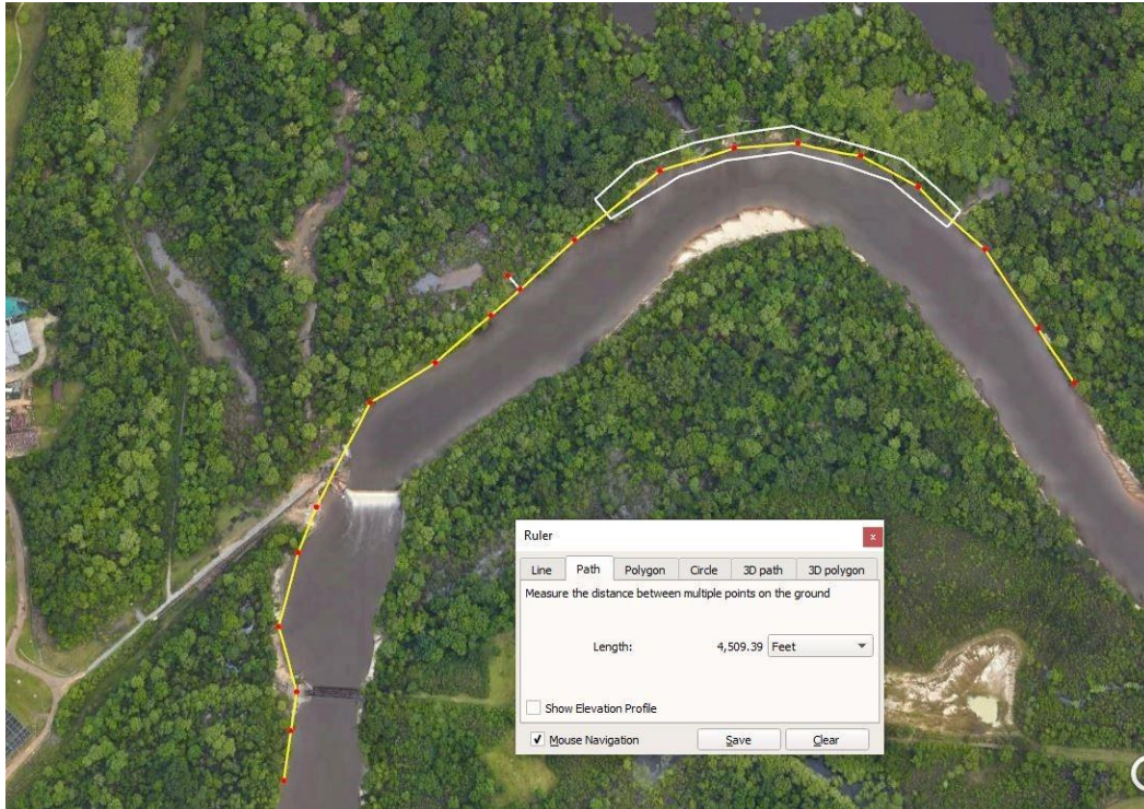
Figure 2-14. Stone Placement West Bank to protect the Fewell Treatment Plant Weir and May's Lake Tie-In
