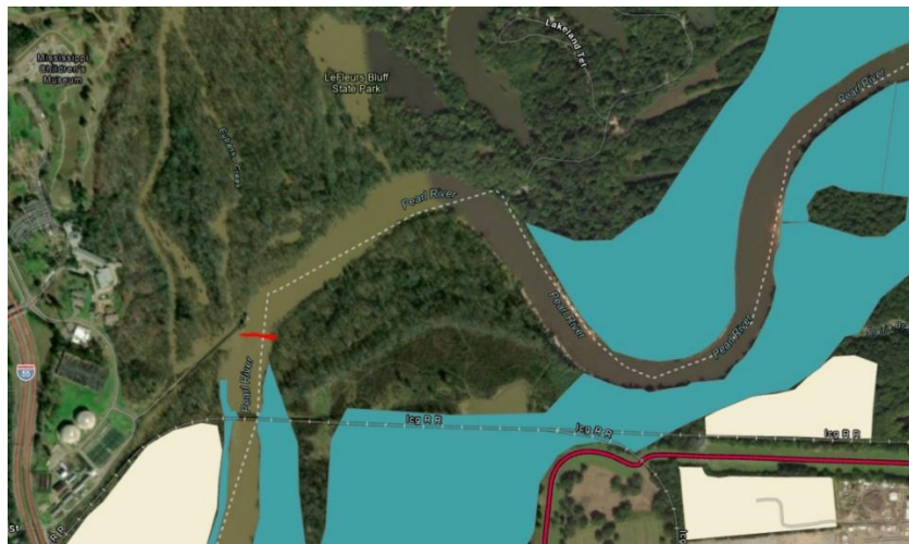
Figure 2-12. Mays Lake and J H Fewell Weir, as compared to the Excavation (blue) and Fill (tan)
