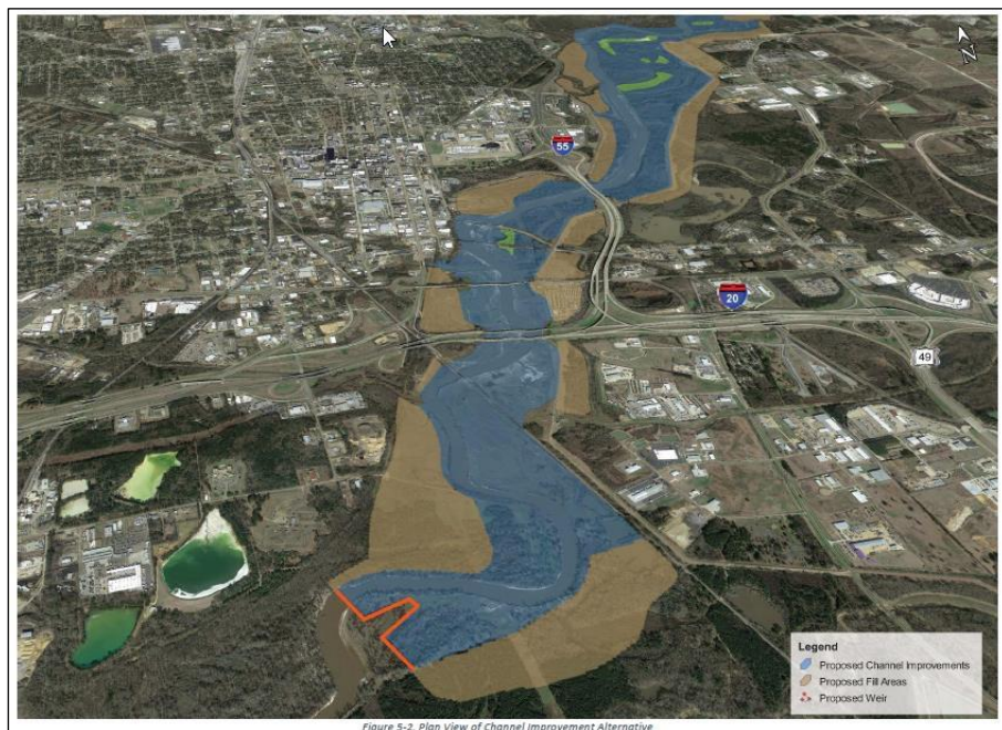
Figure E2-2. Plan View of Proposed Channel Improvements, Excavated Material Plan, & Weir
