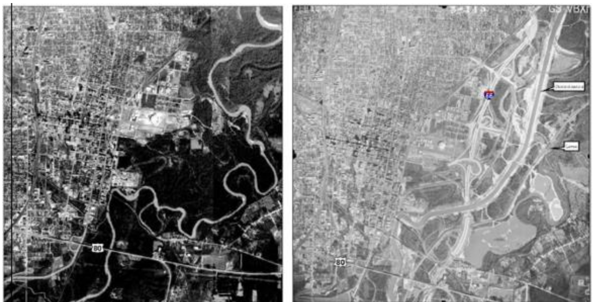
Figure 2-2: Levees and Channel Straightening. (Source: Rankin Hinds 2021)
