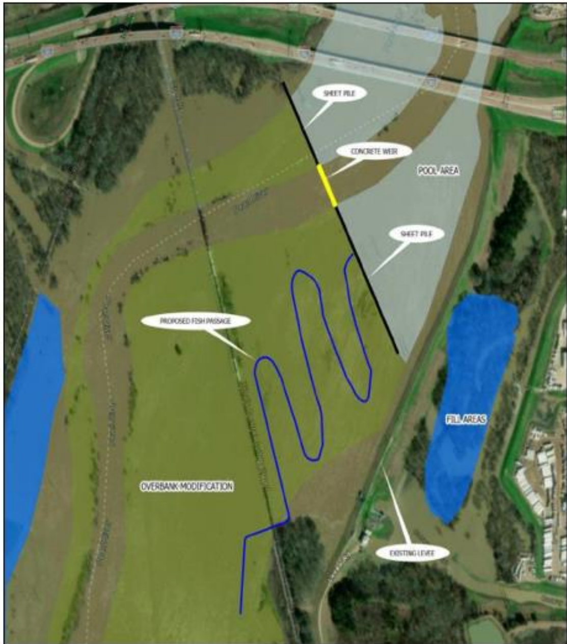
Figure 3-7: Proposed Weir (Black) and Fish Ladder (Blue) Exact Dam Design to be determined in PED
