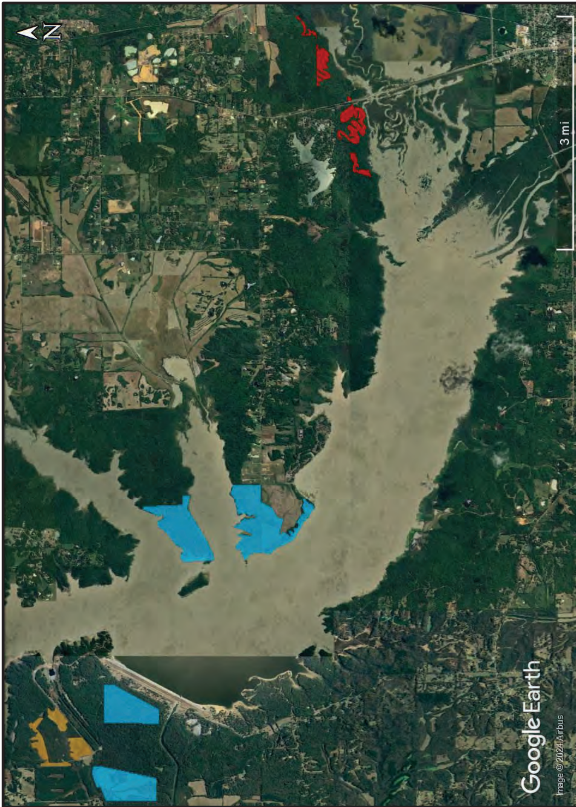
Figure 6. Proposed potential borrow locations (light blue represents clay borrow sources, red represents sand borrow sources, orange represents borrow source locations preferred by lake field office personnel).
