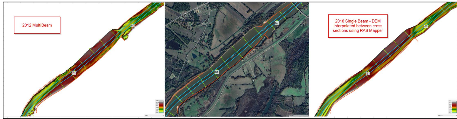
Figure A-124. 2012 Multi-beam versus 2016 Single-beam Cross-Section Comparison (RM 61)
