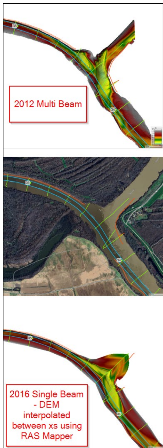
Figure 100. 2012 Multi-Beam and 2016 Single-Beam Data Near RMs 34–35
