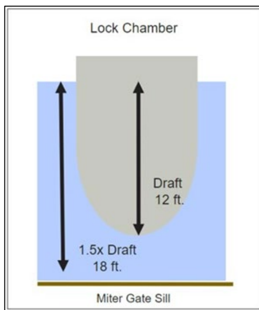
Figure A-139. Lock Chamber Draft Schematic
