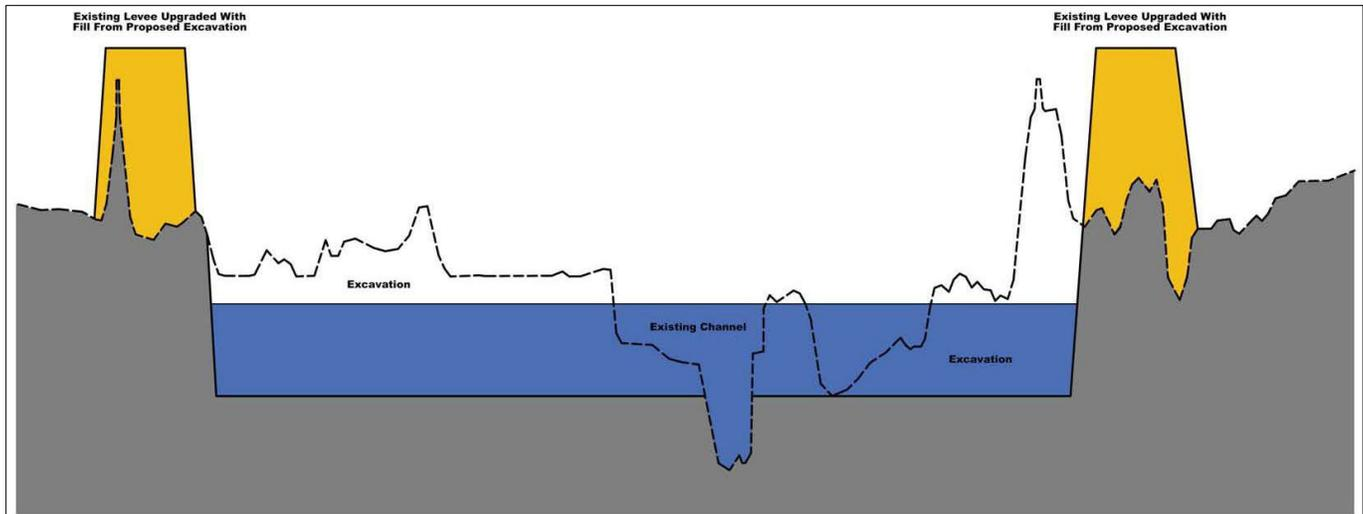
**Figure 7-9.** Channel Improvements with a relocated weir and improvements to existing levees.
