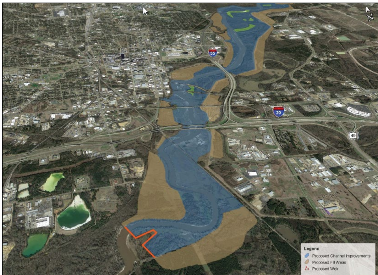
Figure I-5. Plan View of Proposed Channel Improvements Excavated Material Plan, and Weir with Gate
