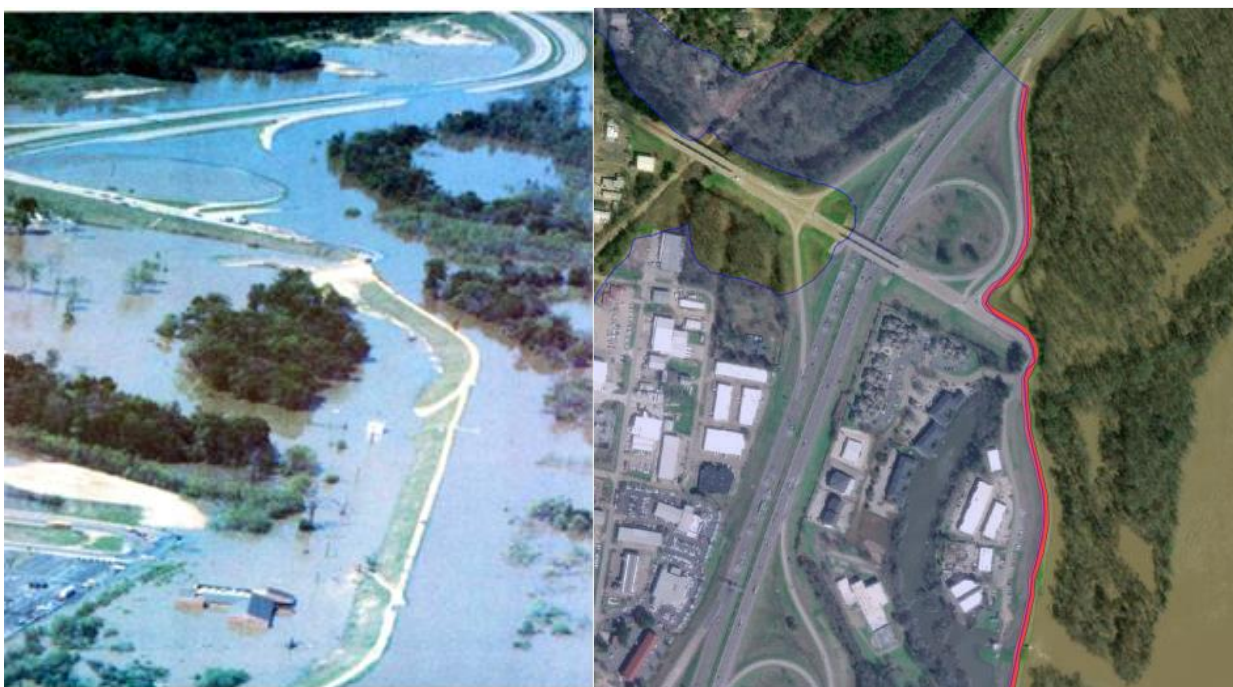
Figure E 2-6. 1984 Levee Extension to Prevent Flanking
