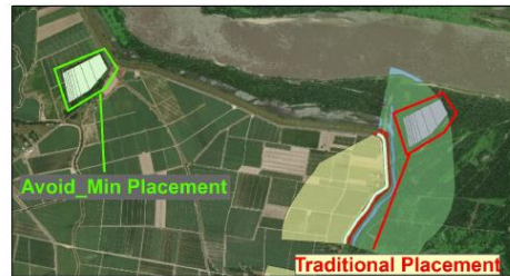
Figure A10-6. Examples comparing Alternative 2 - Traditional Construction with Alternative 3 - Avoid and Minimize at two levee Work Item locations. Note that in both cases, the location of borrow pits were shifted from forested areas on the riverside of the levee to agricultural areas on the landside of the levee. This shift resulted in a decrease in impacts to wetland resources.
