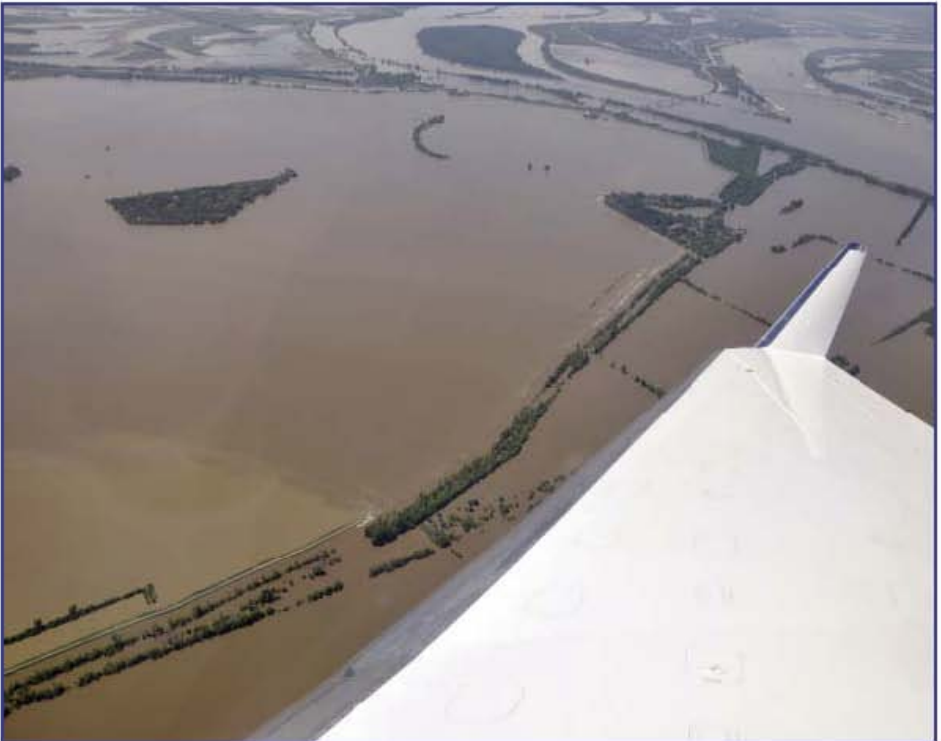
Above: Activation of the lower inflow/outflow crevasse site on May 3, 2011. Below: Aerial view of the upper crevasse site after activation of the floodway.
