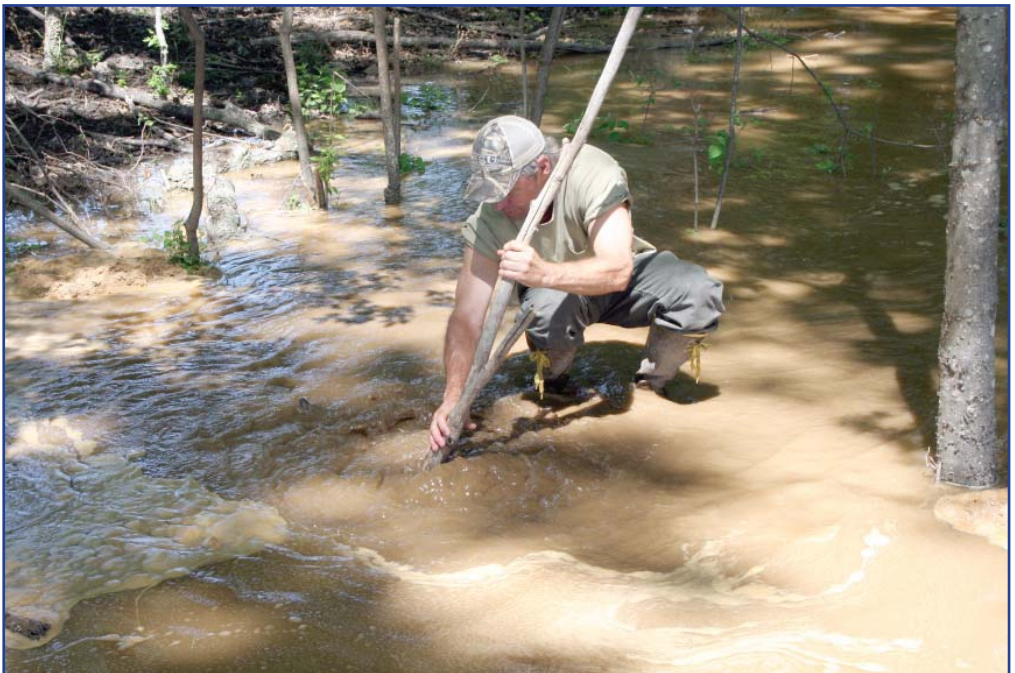
Lanny Barfield checks the high-energy boil at Winterville, Miss.
